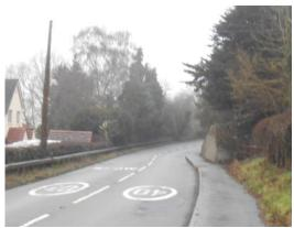
3.10 The existing easternmost 40mph terminal signs are not clearly visible as they are positioned under overhanging canopy of trees (Photo 9), this may impact on the lack of speed reduction after leaving the Ironbridge bypass.
